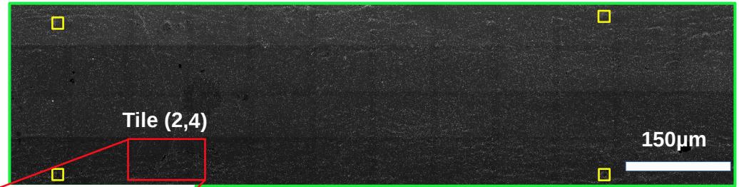
Interrupted in-situ : 2 load steps → \epsilon_p=2.25\%
